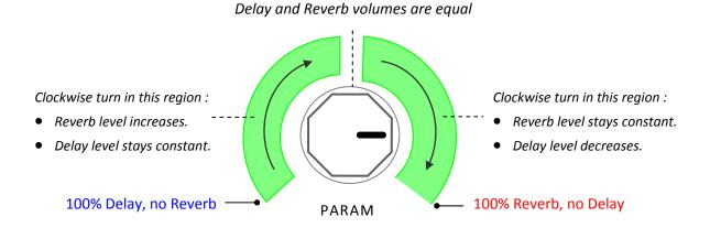
Together with the BLEND knob, you will be able to dial in any desired delay-to-reverb ratio and the overall effect level.
