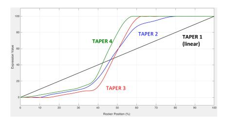
The potentiometers in wah pedals have different taper characteristics, which determines the feel as the rocker sweeps through its sweep range.
